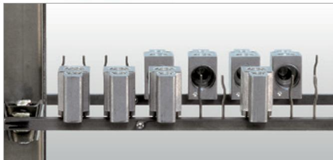
Valve-carrying frame for a complete automatic system with corresponding robotized loading and unloading. The valve-carrying rods work through a bayonet quick locking system. Max tolerance: 0.2 mm.
